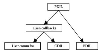
The above diagram shows which DILs know about and use other DILs. The CDIL and FDIL are completely stand-alone; neither requires the use of any other DIL. The PDIL makes extensive use of the FDIL and require its presence. The PDIL can use the CDIL if the application developer desires, but it does so indirectly through the use of application-defined callback functions.
